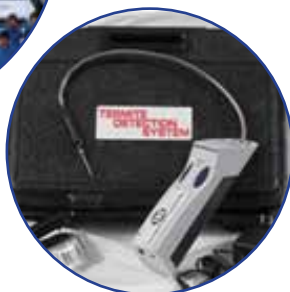
Termite Detection System
